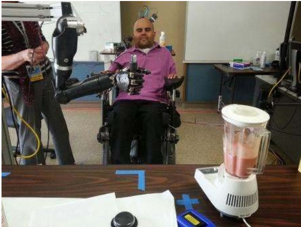
Erik Sorto controlling a grip switch with a robot hand to make a smoothie. Credit: Spencer Kellis/Caltech
