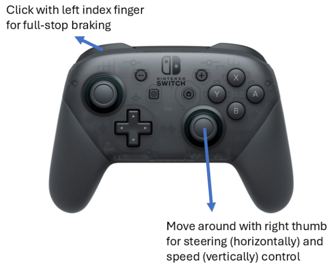
Figure S5: Joystick programmed for the bimanual cursor-and-click driving control of motor intact participants. They used the joystick in the simulated town driving task modified from the CARLA Leaderboard 2.0. The top left button was clicked with the left index finger to trigger full-stop braking of the vehicle. The right thumbstick was moved around with the right thumb to trigger the vehicle's steering value changes horizontally and its speed value changes vertically.
