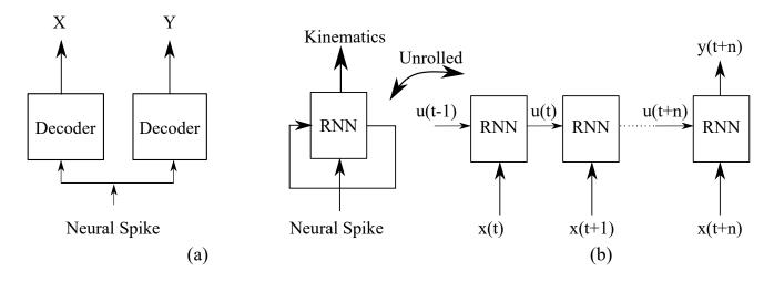
Fig. 3. Output of the decoding algorithm. (a) For the neural network algorithms, two separate decoders are used to predict X and Y position of the cursor. (b) A block diagram of RNN [13] with a single dense layer for regression. Also, an unrolled block diagram of RNN with multiple time-steps. The RNN unit can be either a fully connected SimpleRNN cell or an LSTM unit cell.
