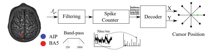
Fig. 2. System architecture for decoding neural signals into relevant kinematics. Broadband recorded data were bandpass filtered (250 Hz - 5 KHz) and thresholded at -4 times the noise RMS. Threshold crossing timestamps were binned in nonoverlapping 50ms intervals and smoothed to estimate the instantaneous threshold crossing rate. Decoding algorithms map these input features to corresponding X and Y coordinates of the cursor on screen.
