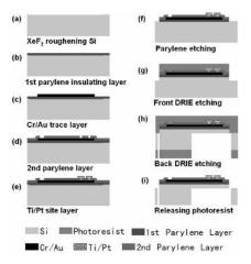
Figure 3. Fabrication process flow.
