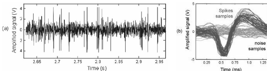
Figure 6. (a) Sample filtered neural data recorded from one channel of the neural probe in rat cortex; (b) Sample action potential waveforms.
