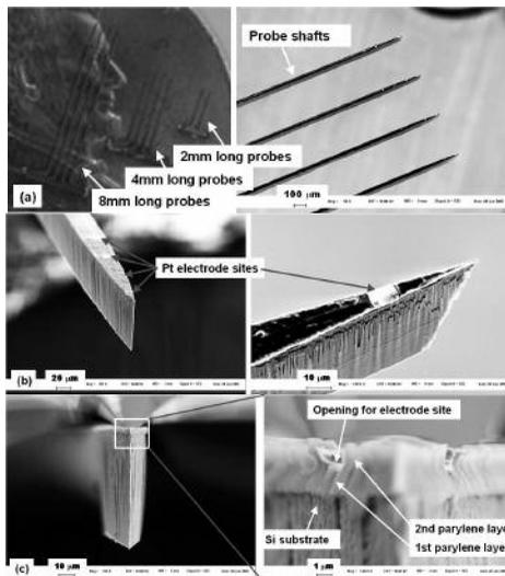
Figure 4. The optical and SEM pictures of the fabricated probes. (a) Pictures of the whole probes and shafts; (b) SEM pictures of the probe tip with multiple electrode sites; (c) SEM pictures of front side view of the probe tip, showing the interface between parylene layer and Si substrate and the interface between two parylene layers.
