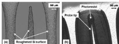
Figure 5. Fabrication process pictures. (a) Roughened Si surface; (b) Photoresist protection for probe tips during back DRIE etching.
