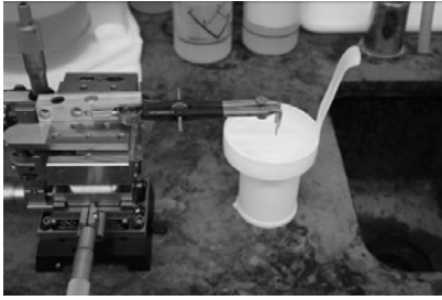
Figure 5. Meniscus etching setup. The probe-only device is pulled out of the silicon etchant by a manipulator located on the left hand side of the picture.
